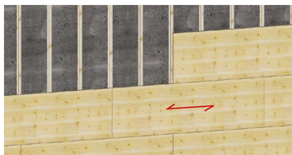
Structure verticale (mur) – pose horizontale
